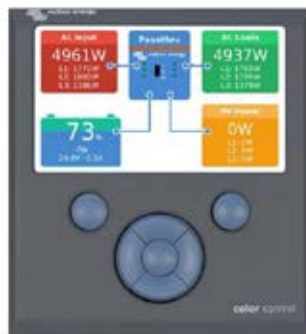
Color Control GX, showing a PV application
